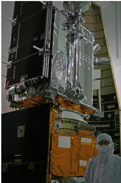
LRO (gray) and LCROSS (yellow) lunar spacecraft stacked adjacent to Atlas V payload fairing at Astrotech Payload Facility on May 15, 2009. Credit: Ken Kremer and the Planetary Society.
