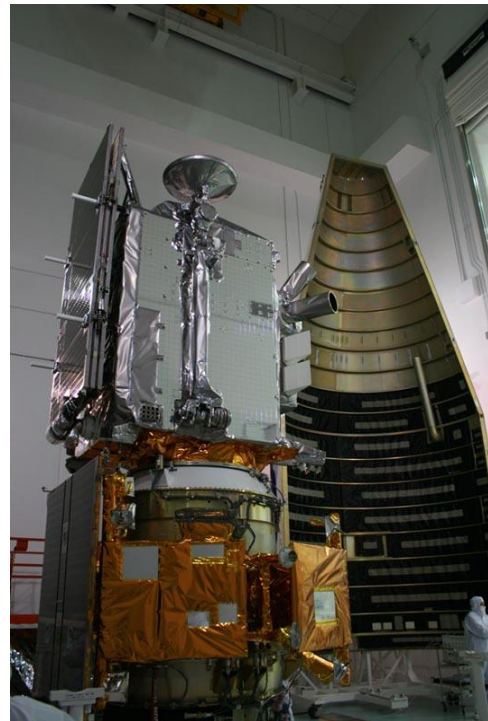
LRO (gray) and LCROSS (yellow) lunar spacecraft stacked adjacent to Atlas V payload fairing at Astrotech Payload Facility on May 15, 2009. Credit: Ken Kremer and the Planetary Society.
