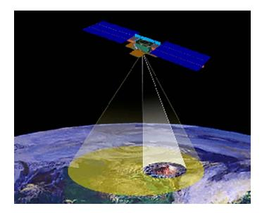
The Autonomous Sciencecraft technology that will be tested as part of ASA's Space Technology 6 mission will use artificial intelligence to select and transmit only the scientifically significant images.
